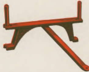
Lateral braces on both bolsters take backward and forward thrust that shortens the life of ordinary wagons.
