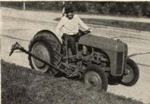
HEAVY-DUTY MOWER. For highway or municipal use. Cutterbar raised or lowered by finger tip control.
