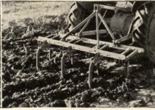
FERGUSON TILLER. All-purpose field cultivator or sub-soiler. Spring-trip resets tines on the "go."
