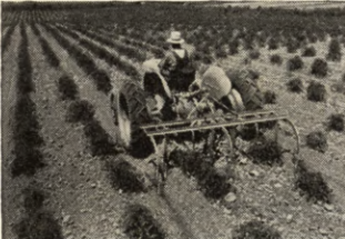
IMPROVED ROW-CROP CULTIVATOR. Two-way adjustable sweeps. Follows front tractor wheels like a shadow.
