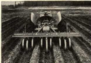
SPRING TINE CULTIVATOR. Can be operated full speed all day in land full of obstructions, without damage.
