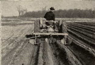
THREE-ROW RIDGER. For potatoes and vegetables. Bottoms adjustable for 24" to 30' rows. Has great strength.
